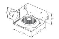
Fan Housing for SLM50 and SLM70
